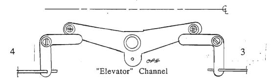
Similarly, when the trigger has moved the elevator portion of the aux. crank so that it is farthest from you, moving the aux. handle to the "up" position will bump yet another 90° crank nearby, and so on, enabling functions Five and Six.
